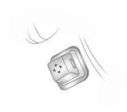
For vehicles with the power tilt wheel, the control is on the left side of the steering column.
